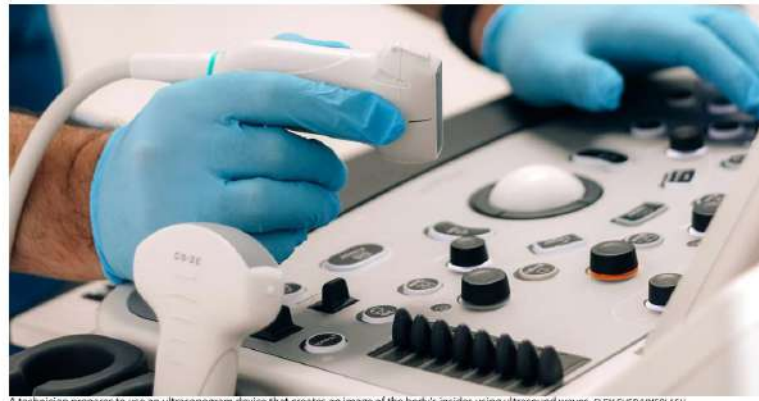
A technician prepares to use an ultrasonogram device that creates an image of the body's insides using ultrasound waves. ELEN SHER/UNISPLASH
