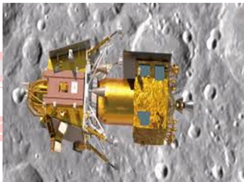
Separation of lander and propulsion module
