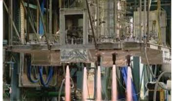
The Indian Space Research Organization successfully flight tested the Service Module Propulsion System (SMPS) of Gaganyaan at ISRO's Propulsion Complex (IPRC) at Mahendragiri, Tamil Nadu. The test consisted of five Liquid Apogee Motors (LAM) (normal rocket engines) each with 440 Newton thrust and 16 Reaction
